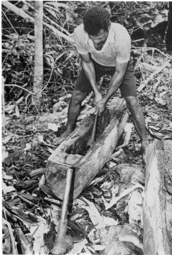
Fig. 9: With the interior well established, the hole-tanged adze ( tabumagimagi ) is used to form the bottom of the trough.
