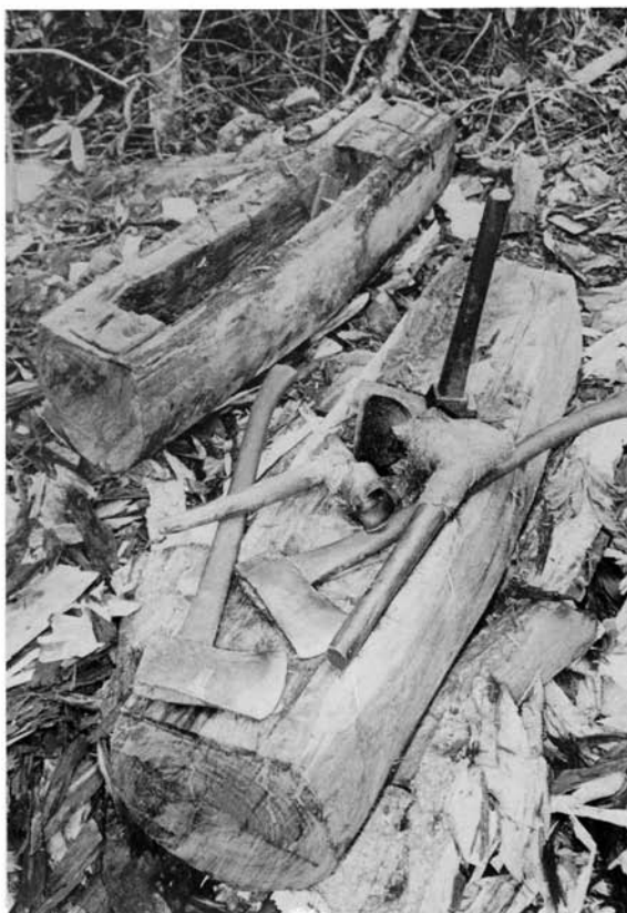
Fig. 4: Two lali in progress, with the craftsman's tools displayed. In order away from the viewer these are: 1 & 2, Felling axes - vulaono ; 3, adjustable gouge-adze - cālocālo ; 4, broad-axe hafted as an adze - valevatu ; and 5, hole-tanged adze - tabumagimagi .
