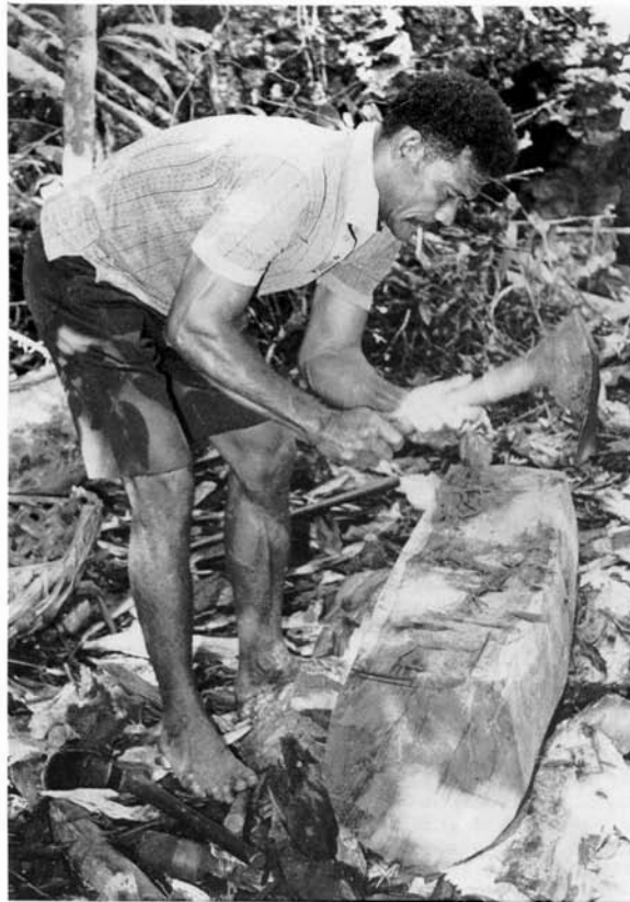
Fig. 7: Beginning the tuki dreke - chopping out the interior of the lali . The valevatu is being used to 'set out' the shape of the cavity. The offset form of the edging-axe blade is evident in this photograph. As can be seen, the flattening of the top of the lali ( cicikete ) has been completed and the outside shape has also been established ( umani ).
