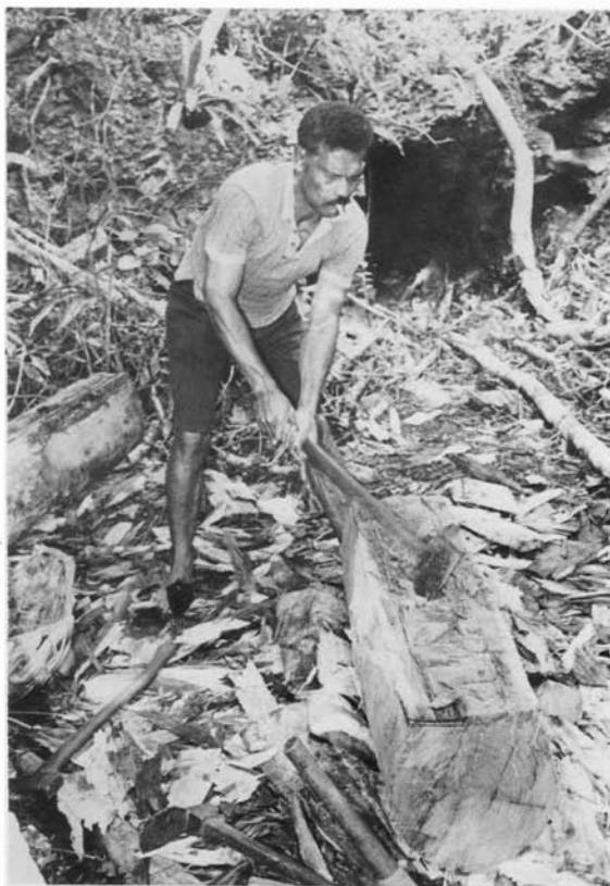
Fig. 8: Continuing the tuki dreke with the felling-axe.
