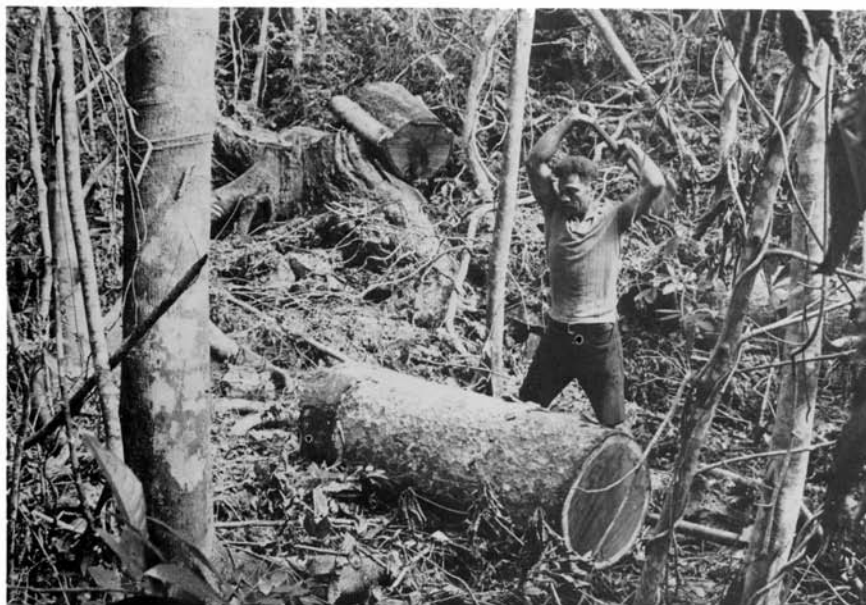
Fig. 3: Beginning the flattening - cicikete - of the top ( ketena ) of the lali . The stump of the parent vesi can be seen in the background, with its roots growing round a limestone outcrop.
